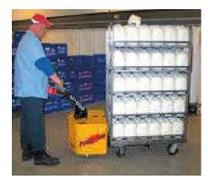
The **Power Tug**<sup>™</sup> is designed to promote productivity with minimal manpower by mobilizing up to 5,000 pounds with ease. It has a mono-drive wheel with a stabilizing swivel caster that enables the unit to mobilize loads over uneven surfaces with complete control. It's body equipped with an electric actuator accomodates various lead heights.
