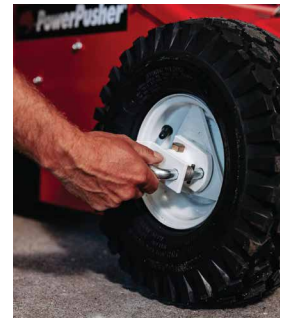
Free Wheeling Hub (Standard on Automotive PowerPusher models)
