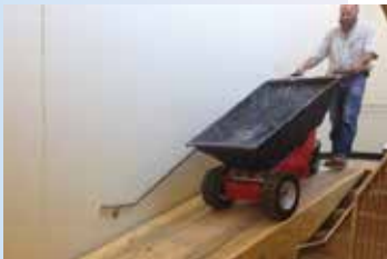
The Power Pusher electric wheelbarrow can easily be pushed, pulled and lifted by only one operator.
