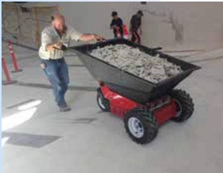
The Power Pusher electric wheelbarrow eliminates the pushing, pulling and lifting required with other wheelbarrow solutions.
